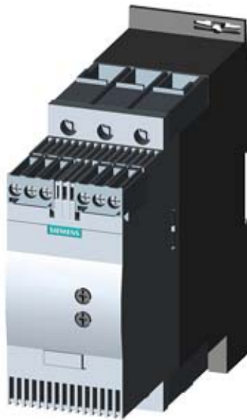
SIRIUS SOFT STARTER, SIZE S2, 72A, 37KW/400V, 40 DEGREES, 200-480V AC, 110-230V AC/DC, SCREW TERMINALS
